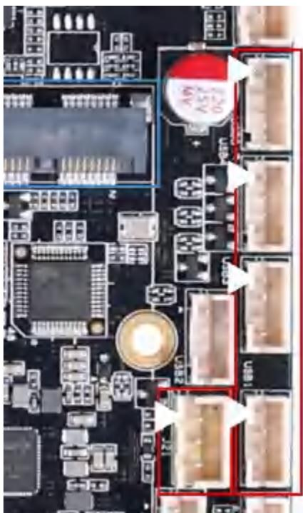
The board has 5 USB2.0 sockets for peripheral expansion, the default is HOST, and the power supply current of each channel is not more than 500mA. Among them, USB5 is directly output from CPU, and others are converted from USB HUB.
