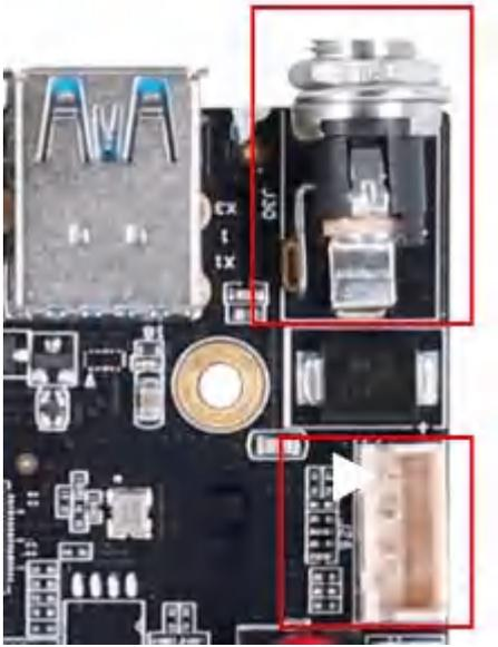
The interface of the power socket is defined as follows, the power board can be used for power supply, and the socket specification is 4PIN 2.54mm pitch.
