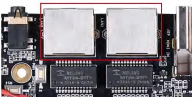
The board supports 2 Gigabit Ethernet ports.
