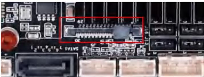
The board supports a 1300W pixel MIPI camera, and the electrical definition of the socket is as follows:
